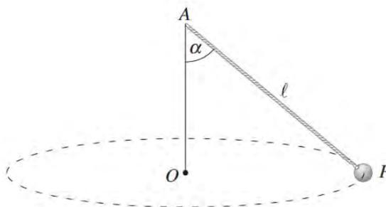
The forces acting on the particle are the tension,  $T$ , in the string and the force due to gravity,  $mg$ .
